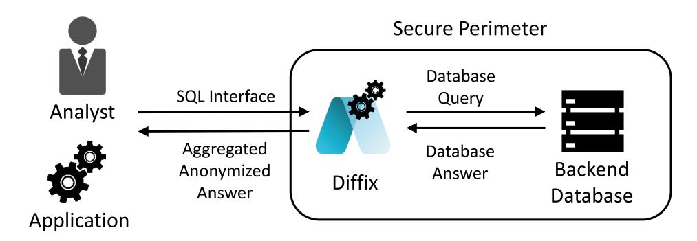
Deployed as a "box" in front of an unmodified (raw) database
